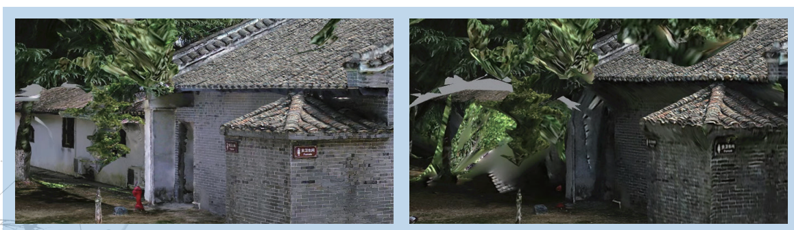
Comparison of the model of the part of Huang Xing's former residence behind the house obscured by trees (The left is the result of the 3D model after fusing drone and Hi-Target vRTK data The right is the result of the 3D model from UAV tilt photography) FIG9
