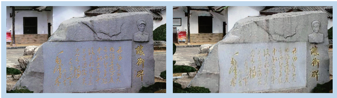
Comparison of the model of the former residence of Xu Guangda to let the title monument (The left is the result of the 3D model after fusing drone and Hi-Target vRTK data The right is the result of the 3D model from UAV tilt photography) FIG10
