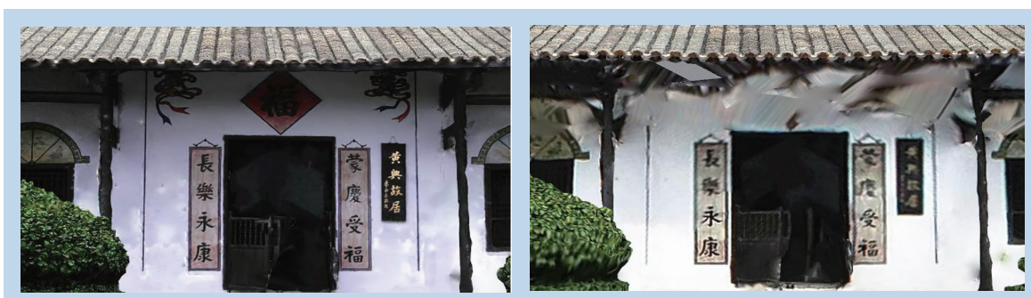
Comparison of the front elevation model of Huang Xing's former residence (The left is the result of the 3D model after fusing UAV and Hi-Target vRTK data The right is the result of the 3D model from UAV tilt photography) FIG8
