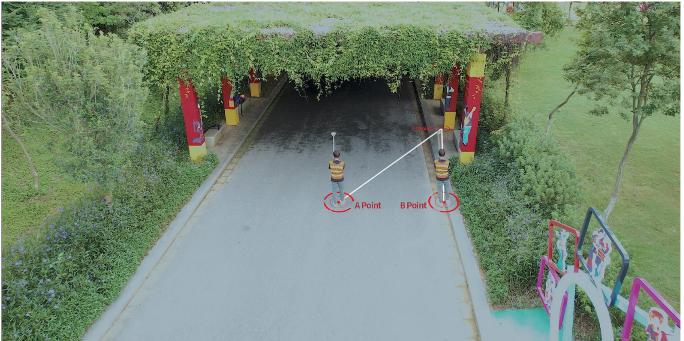
AR Measurement by RTK GNSS Receiver FIG3
