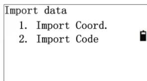
As an example of importing coordinate data, press [1] yo enter the interface of “Select file”. The files in the directory of “PROJECT” in U disk will be read.
