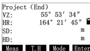
Press [Meas] to start measuring, then you can press [Enter] to return to “project” menu and press [3](Project)(3.Project) to start projection measurement.
