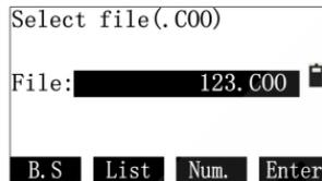
You can input the file name used to save the received data, such as “123”(COO). If the file exists in the instrument, prompts “File Exist”. If selecting [List], you can select a file in FLASH disk. After selecting file, press [Enter] to enter the interface of importing;
