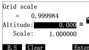
After input altitude, you can press [Enter] to calculate the “Scale”,as shown in the picture above. Press [ENT] to save the scale grid and exit this interface. Exceptions:
