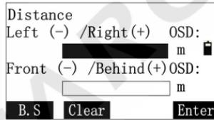
The relation between “+” and “-” is referred to the diagram of angle offset. After input the known distance, press [ENT] to enter the interface of “Offset (dist1)-Prism”:
