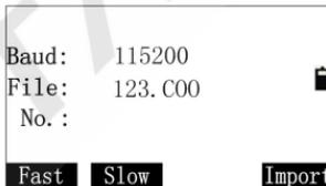
The only column that can be set is the Baud. The Baud available are 2400, 4800, 9600, 19200, 38400, 57600, 115200 with respect to the RS232C serial communication bus. The bauds can be set with soft keys [Fast] and [Slow]. Usually, 115200 Baud is adequate for importing.
