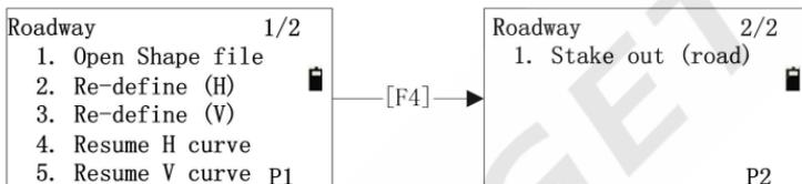
If you have already imported [.LS] files into the instrument from the external, you may open the [.LS] file through ‘1.Open Shape file’. You can choose the three opts after opening the LS file: ‘Stake out (road)’, ‘Resume H curve’ or ‘Resume V curve’.
