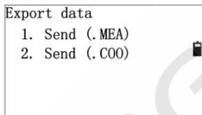
Taking an example for measured data, press [1] to enter the next interface, you need to input the measurement file you want to export or press [F2] to retrieve.(you may not input extension ,the file when exported will defaults it’s format as “.MEA”);
