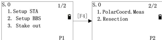
The ‘Setup STA’ and ‘Setup BBS’ are the preparation work for staking out. If you have already setup them, re-setting them are not necessary.
