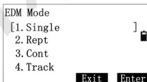
Press [▲] or [▼] to move the “>” to the options needed, then press [Enter] to receive the select, and save it to system file. After shut on the instrument next, the mode defaults as the selected mode. The other settings are same as “EDM Mode”, not tired in words here.
