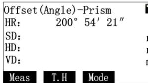
If you want to re-input the target height, press [T.H] to re-input. Press [Meas] to start measurement. After measuring, press [Enter] to enter the interface of “Offset (angle)-Result”:
