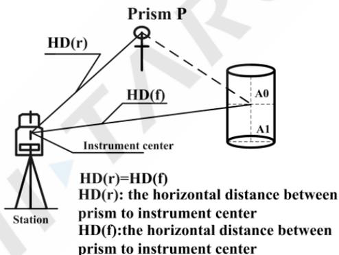
When measuring the coordinate of the earth point ‘A1’ which is the projection of ‘A0’, set up the height of instrument and the height of target.
