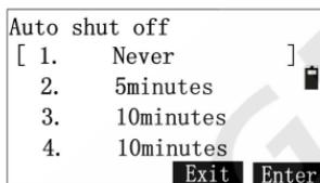
You may choose ‘Never’ to cancel the auto shutdown. When choosing 5, 10, 20 minutes opts, the instrument will shut down automatically if there is no key pressed. Use the [▲] or [▼] keys to move indicator ‘[]’ up and down to the option wanted. Press soft key [Enter] or [ENT] to save the setting. Pressing [ESC] will result in no changes of settings.
