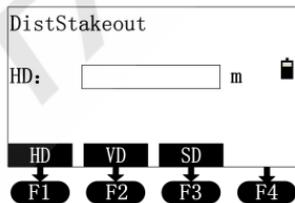
The keys [F1]->[F3] is to select the stakeout mode. After select the mode, input distance (HD), then press [Enter] to enter the distance stakeout mode, and you can press [F2] to get the result of stakeout.
