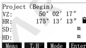
Press [Meas] to start measuring, then press [Enter] to enter the interface of “Project(End)”;
