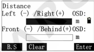
The relation between “+” and “-” is referred to the diagram of angle offset. After input the known distance, press [ENT] to enter the interface of “Offset (dist1)-Prism” :
