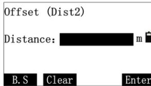
Input the distance, and press [Enter] to enter the interface of “Offset -Begin”. You must aim at point “P0” to measure. After measuring, press [ENT] to exit the interface to enter the interface of “Offset-End”.
