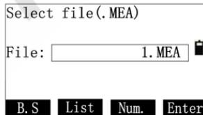
After selecting the measured file, press [Enter] or [ENT] to enter the interface of “Select format”. **The format of “Sunway” that the transmission software our instrument equipped can receive and analysis. But the format of “SSS” means the format of Topcon (GTS-7), which you can’t use the t transmission software our instrument equipped to receive. You must use “Topcon link” software or other can recognize**
