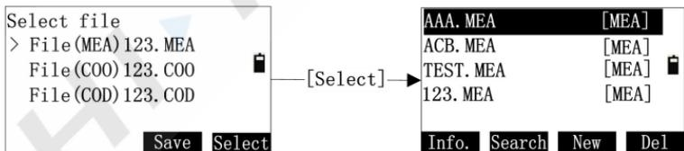
Use [▲] or [▼] keys to move indicator ‘>’ to the wanted type of the file and press [ENT] soft key to enter the File list as shown above.
