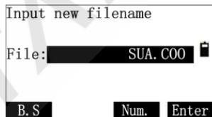
The filename extension of imported file will be changed as “.coo” automatically, which is the standard coordinate filename extension in instrument. Input the new filename after importing, and press [F4].
