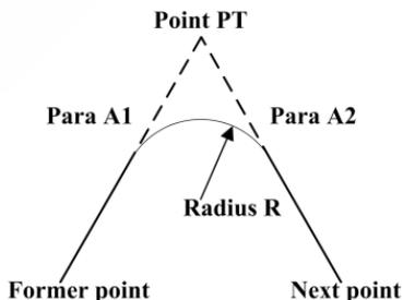
‘PT’ is the intersection point of road. The ‘x’ of ‘Px’ is the number of intersection point.
