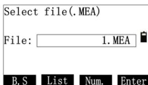
3) After selecting measurement data, press [F4] to enter the interface of “Input new filename”, which defaults the selected file with with “.txt” extension;
