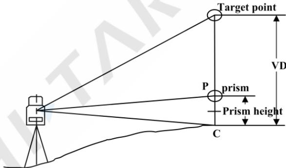
There are two modes for 'REM' measurement: 'Input TH' and 'without TH'. You can select 'Input TH' mode when you need the altitude from ground to target, otherwise 'without TH' when you need the altitude from any reference point to target.
