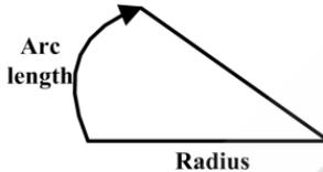
The value of Radius (R) can be negative. The positive direction is the right direction along the designed roadway, and the left is negative. The “Len.” refers to Arc length.
