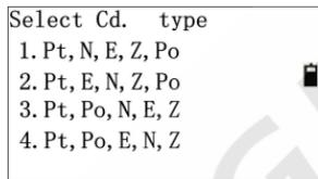
Select the coordinate format matched coordinate file, such as ,if the file “SUA.TXT” selected is saved according to the “Pt,N,E,Z,Po”, you can press [1] to enter to the next interface;
