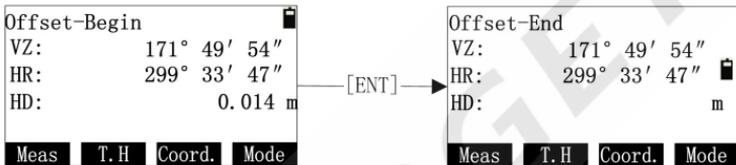
Aim at the end point, and press [ENT] after measuring. The coordinates of measured points are displayed, as shown in picture below:
