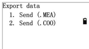
2) AS an example of measurement data, press [1] to enter to the next interface, as shown in picture below. Input the measurement file which needs to be exported or press [F2] to
