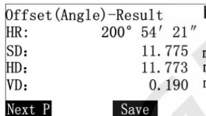
Then, aim at offset point, you can get its coordinates. Pressing [Next P] to measure next point; press [Save] to save the coordinates of offset point; press [ESC] to exit.
