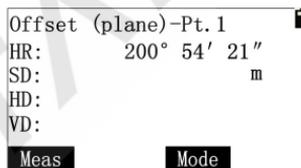
Press [Meas] to measure point 1, and press [Enter] to receive the measured data and enter the interface of "Offset (plane)-Pt.2". Refer to the operation of measuring point 1 to get the data of point 2 and point 3 to enter the interface of "Offset (plane-Result)";
