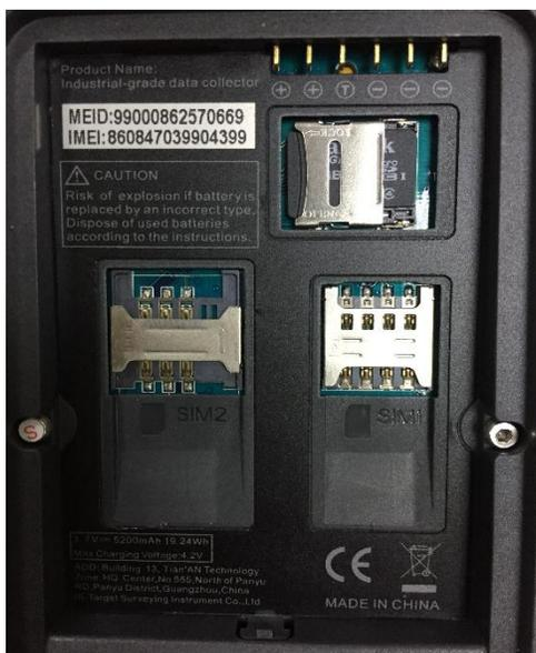
Figure 9-4-9 Installation of SIM card
