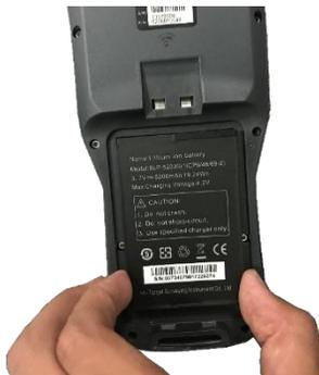
Figure 9-4-4 Dis-assembly of the battery
