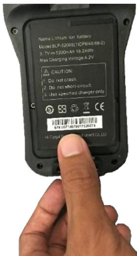
Figure 9-4-3 Installation of the battery
