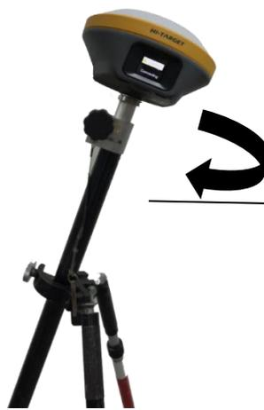
Unscrew the knob and hold the pole to rotate device clockwise slowly around pole.
