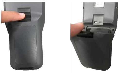
Figure 9-4-7 Battery cover Figure 9-4-8 Lock the battery cover
