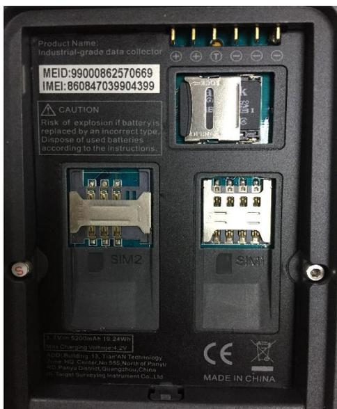
Figure 9-4-9 Installation of SIM card
