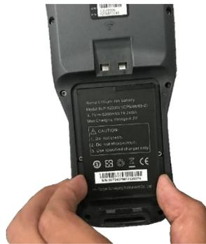
*Figure 9-4-4 Dis-assembly of the battery*
