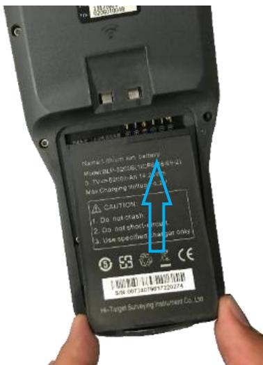
Figure 9-4-2 Installation of Battery
