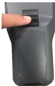
Figure 9-4-6 Lock the battery cover
