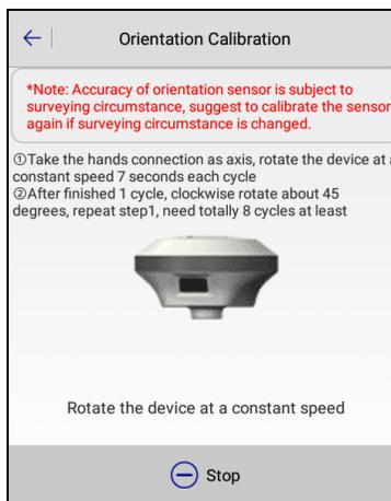
Figure 7-1-12 Rotate The Device
