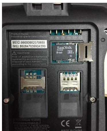
Figure 9-4-14 Installation of Micro SD card
