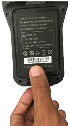
*Figure 9-4-3 Installation of the battery*
